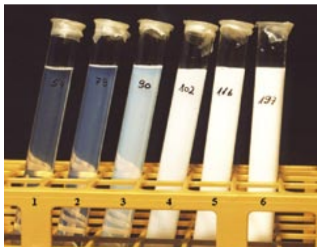
Figure 5: Correlation between particle size and transparency. 1: 54 nm, 2: 79 nm, 3: 90 nm, 4: 102 nm, 5: 116 nm, 6: 197 nm.
