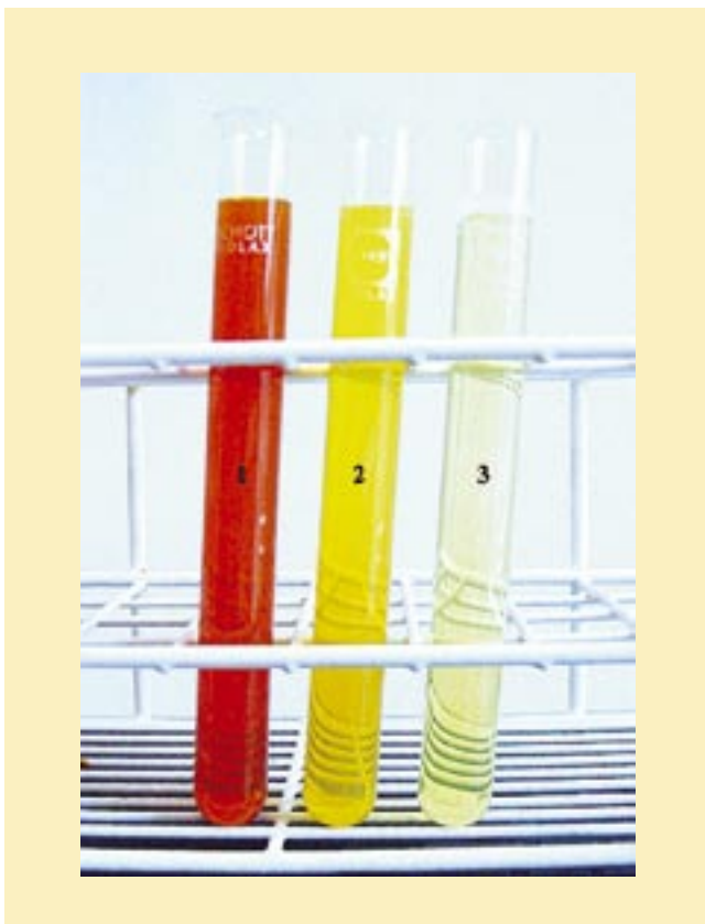
Figure 4: Nanoemulsions containing CoQ10. 1: 7% CoQ10, 2: 0.7% CoQ10, 3: 0.07% CoQ10. The droplet size of all preparations is around 50 nm.
